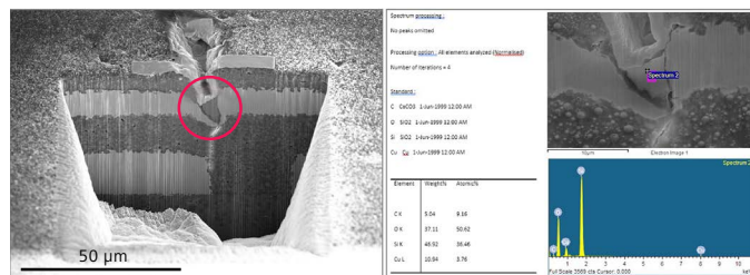
Figure 10 FIB cross-section at the anomalous location showed a sharp-edged particle pressed into the package, cutting open the Cu trace underneath. EDX analysis showed the particle to be a piece of SiO 2 .
