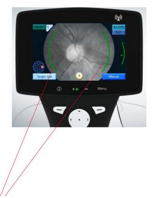
Carefully push the trigger when the two focussing aid lines turn from red to green Structures of the retina, e.g. optic disc and main blood vessels are visible depending on where the fixation target is set.
