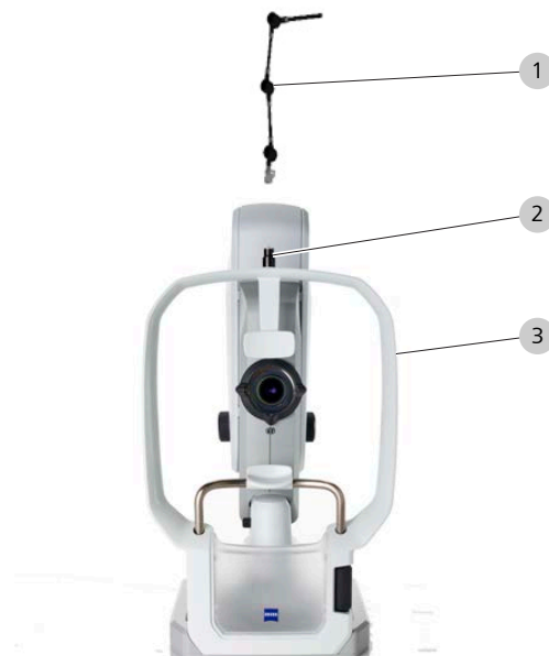
Figure 5: Installing the External Fixation Target
