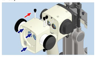
9. Tighten the integrated screws of the beam splitter handtight.
