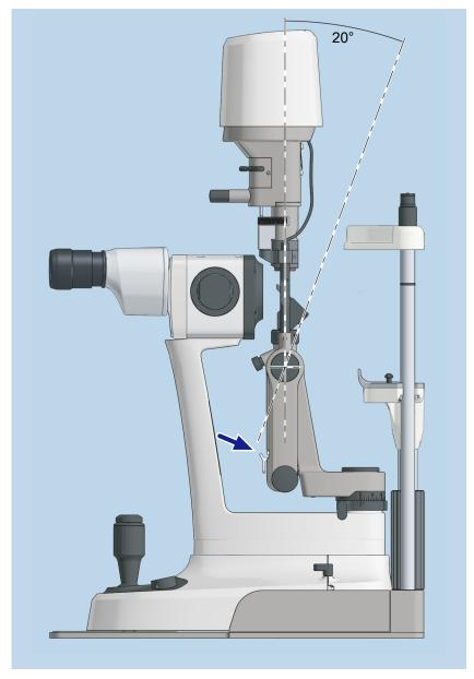
Figure 15: Adjusting the vertical inclination angle (angle of incidence)
