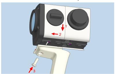
15. Tighten the screws with the size 5 screwdriver, supplied.
