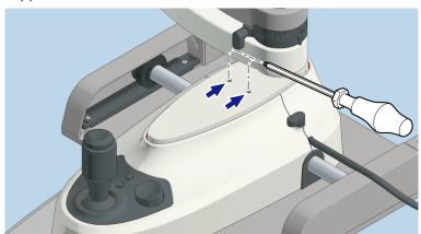
✓ The weight compensation is set correctly when the forces required for the upward and downward movements are balanced in the middle range of the height adjustment.
