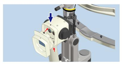
7. Attach the tube adapter 20° by tightening the threaded pin.
