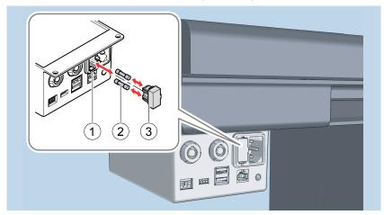
Figure 18: Replace the fuses
