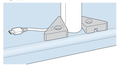
Figure 10: Position the deflectors laterally to the head rest feet on the patient's side of the examination unit.
