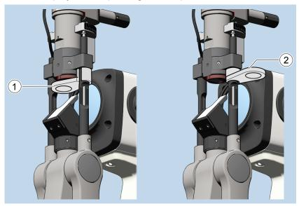
Figure 14: Possible positions of the diffusor on the mirror
