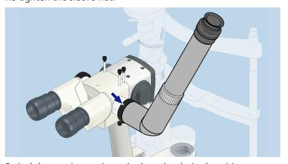
5. Swivel the co-observation tube into the desired position.
