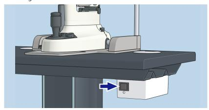
Figure 13: Switching the device on
