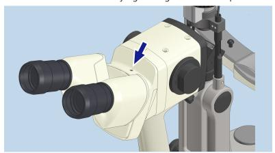
⇒ After successful attachment, the binocular tube must be flush with the tube adapter 20°.
