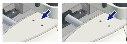
Figure 19: Instrument base with fixed (left) and released (right) springs
