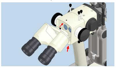
11. Attach the binocular tube to the beam splitter by tightening the threaded pin.
