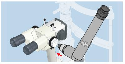
4. Re-tighten the sleeve nut.
