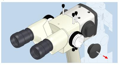
3. Insert the co-observation tube into the attachment. Ensure the appropriate orientation of the co-observation tube is still correct.
