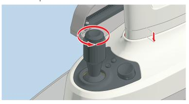
2. Swivel the observation and illumination unit to the side. As a result, two openings become visible, behind each of which there is a screw.
