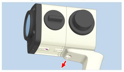
14. Lift the observation unit slightly and position it so that the screw is below the VarioView fundus. **NOTE! Make sure not to kink the cable of the stereomicroscope.**
