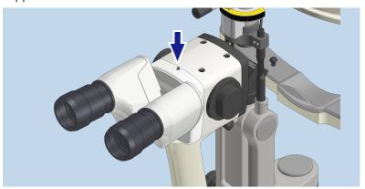
4. Tilt the binocular tube downwards out of the convenience interface.
