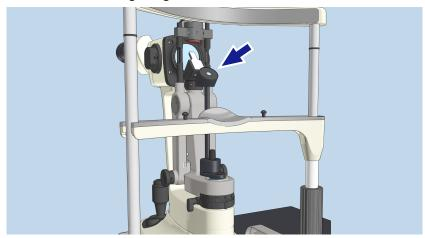
Figure 21: Device with wide-field illumination
