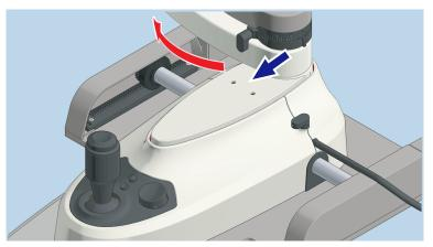
3. Loosen or attach the three screws with the size 3 screwdriver supplied.
