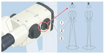
Figure 24: Beam path of Fundus VarioView switched off (A) / on (B)
