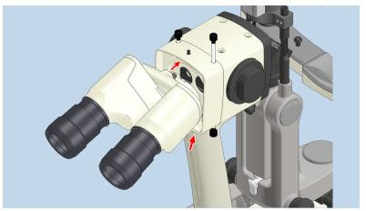
10. Attach the binocular tube to the convenience interface of the yellow filter aperture module by tightening the threaded pin using the size 1.5 screwdriver.
