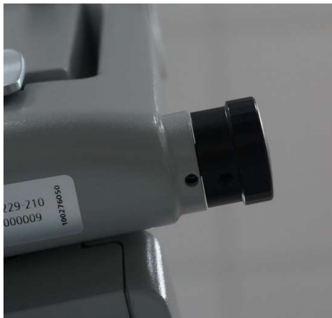
Figure 1: Close-up view from bottom on to right (doctors view) SL 800 slit width control. Of interest is the hole in the main grey part next to the black knob
