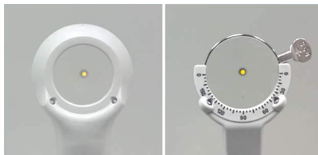
Image 2: The Liquid Trial Lens in comparison to the manual trial lens holder. The aperture of the Liquid Trial Lens on the front side is approximately 28mm and 34mm on the back side. The manual trial lens holder has an aperture at the front and the back of 34mm. In both lens systems, it is the back aperture that limits the field of view.
