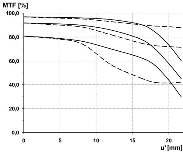
The Modulation Transfer (MTF) as a function of image height ( $u$ ) and slit orientation (sagittal, tangential) has been measured with white light at spatial frequencies of  $R = 10, 20$  and  $40$  cycles/mm.
