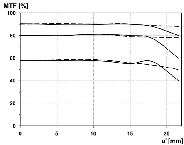
The Modulation Transfer (MTF) as a function of image height ( $u$ ) and slit orientation (sagittal, tangential) has been measured with white light at spatial frequencies of  $R = 10, 20$  and  $40$  cycles/mm.
