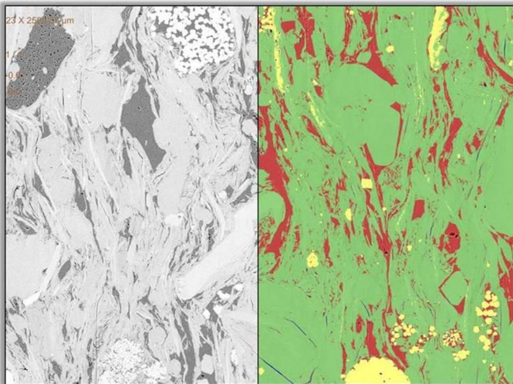
*Figure 1 Large area electron microscopy map, classified using a machine learning algorithm, showing organic hosted pore structures (red), silicate mineral phases (green), pyrite (yellow) and microfractures (blue).*
