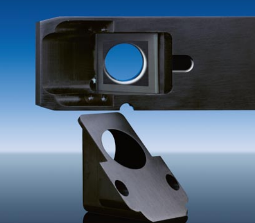
At the front of the laser manipulation slider there is a beam combiner, e.g. 20/80 (epifluorescence/laser). This can be easily exchanged, e.g. for a special beam combiner of the user or a 100% mirror.
