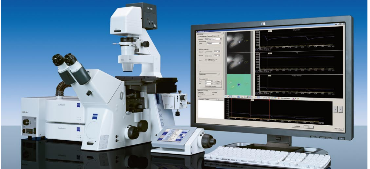
DirectFRAP Imaging System with incubation based on the Incubator PM S1.
