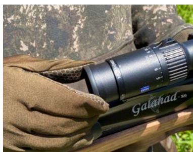
LEFT: There's a massive range of adjustment on the ocular focus ring
